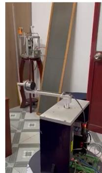
Fig. 11. The inverted pendulum is in upright position (equilibrium point) with CPBCLQR controller which is captured from experimental video. Source: Combining Passivity-Based Control and Linear Quadratic Regulator To Control RIP. <https://www.youtube.com/shorts/JibxqHhBQA4>.
