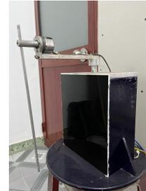
Fig. 10. Rotary inverted pendulum is in idle time.
