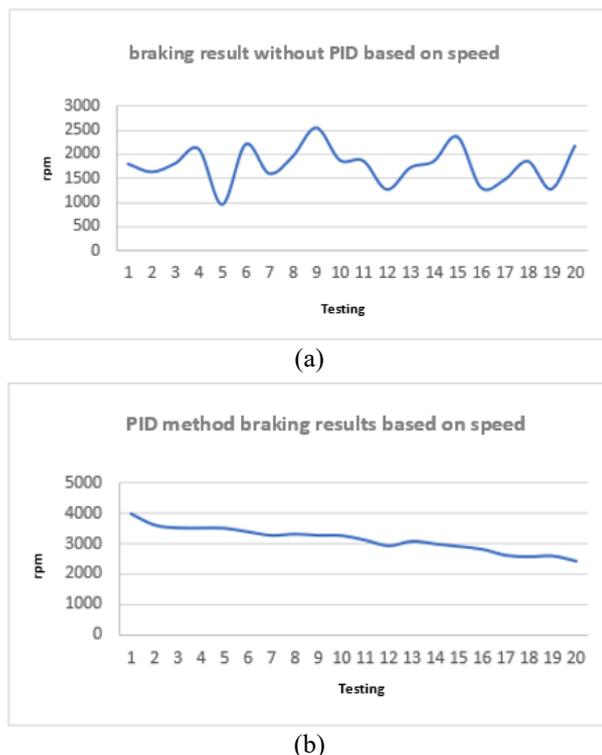
Fig. 28. (a) Results of braking without PID and (b) Results of braking with the PID method
