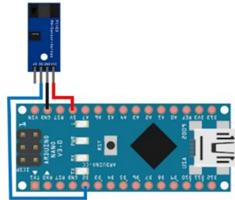
Fig. 10. Rotary encoder sensor pin circuit
