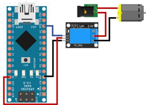
Fig. 11. DC motor pin circuit
