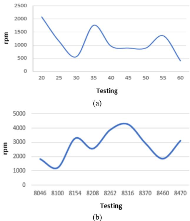
Fig. 17. The results of the two PID tuning tests (a) Graph of results at distance and (b) Graph of results at speed
