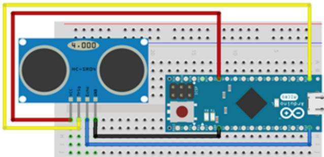
Fig. 9. HC-SR04 ultrasonic pin circuit
