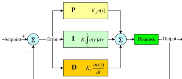
Fig. 1. PID block diagram
