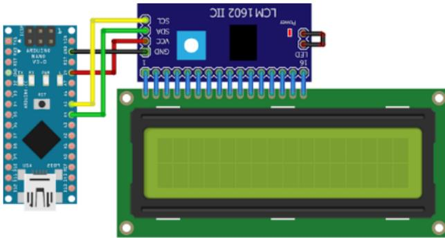
Fig. 8. LCD pin circuit
