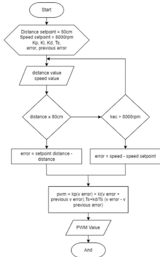
Fig. 14. PID control flowchart
