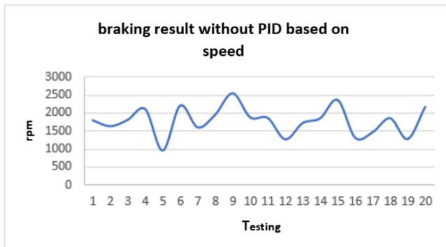
Fig. 21. Graph of test results without PID based on speed
