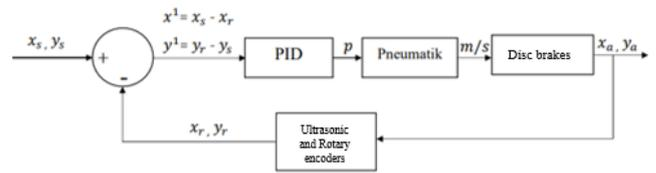
Fig. 7. Braking system block diagram
