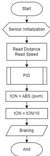
Fig. 13. Automatic braking system flowchart
