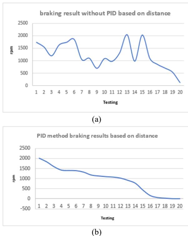
Fig. 27. (a) Braking results without PID and (b) Braking results with the PID method
