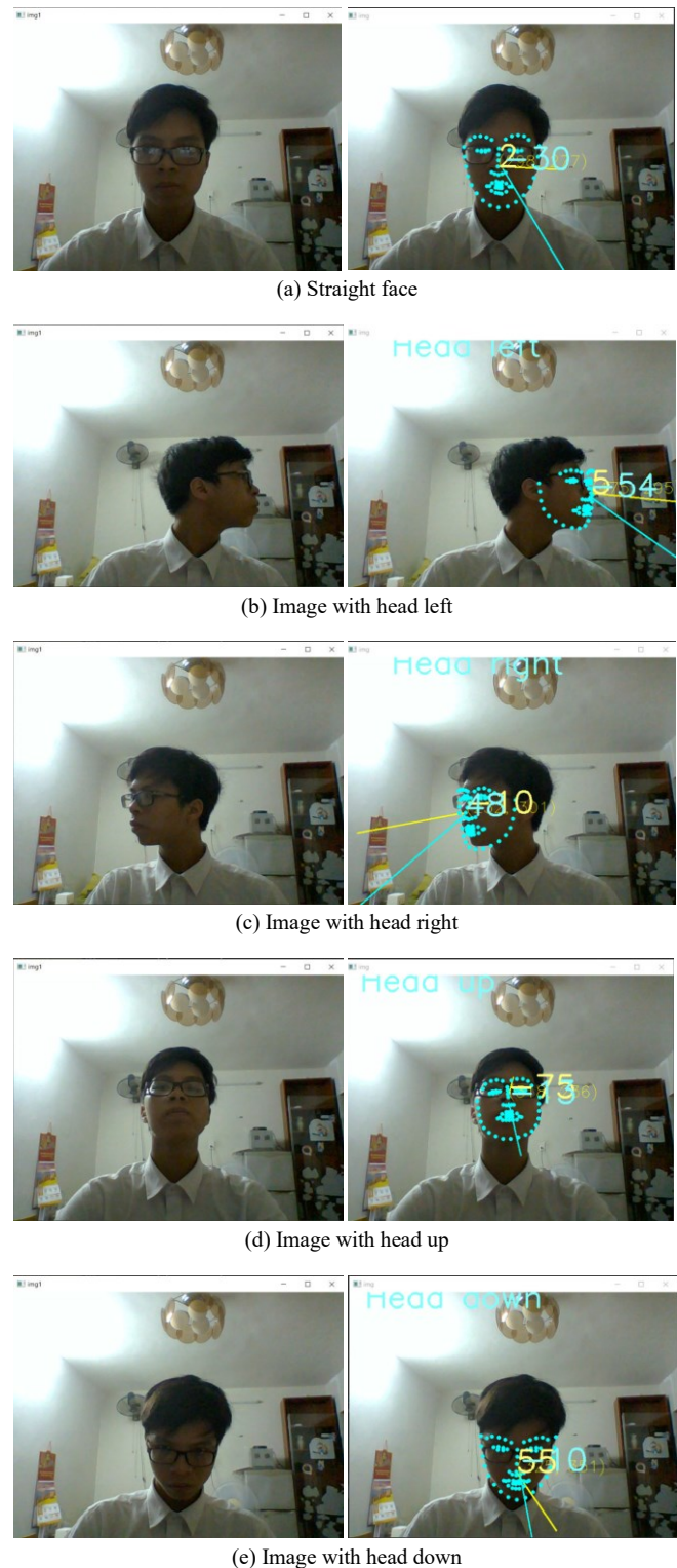
Fig. 7. An example of checking of the different poses of an user ((a) straight face, (b) with head turn left, (c) right, (d) up and (e) down)
