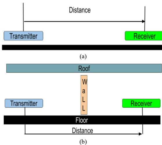
Fig. 6. System testing scheme with horizontal LOS case studies (a) Without Obstacle (b) With Obstacle
