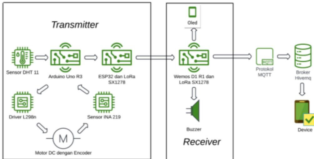
Fig. 1. Lora Transmitter and Lora receiver communication scheme
