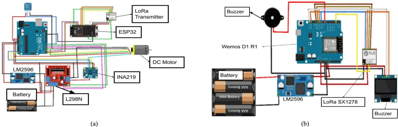
Fig. 2. The Hardware scheme of (a) LoRa Transmitter (b) LoRa Receiver
