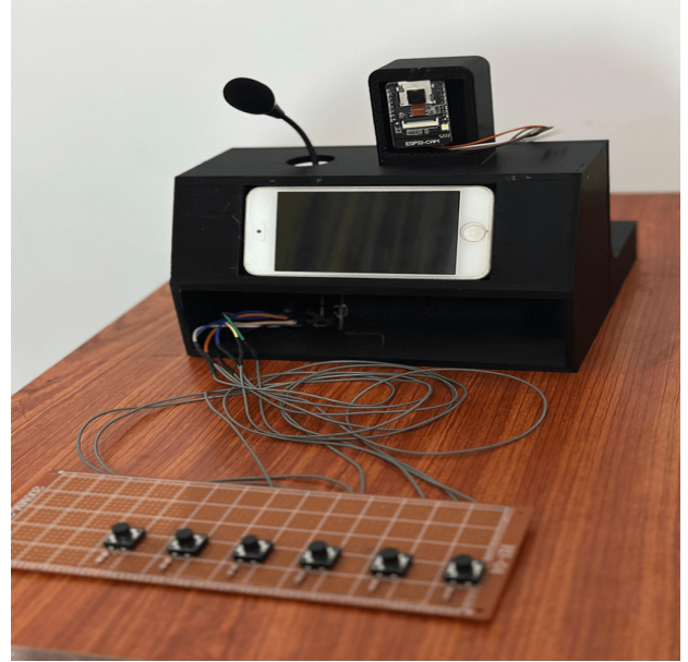
Fig. 14. Prototype of the Communication Device with Braille Keyboard
