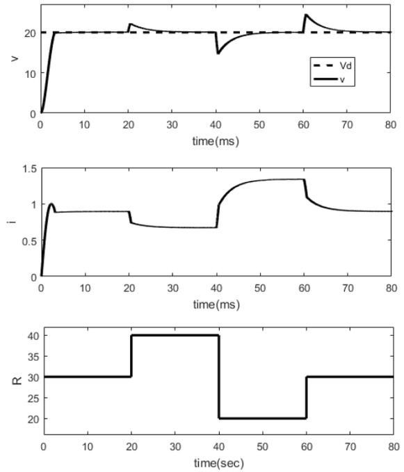
Fig. 7. The results of the SMC when  $R$  changes: the capacitor voltage  $v$  and inductor current  $i$  and load resistor  $R$
