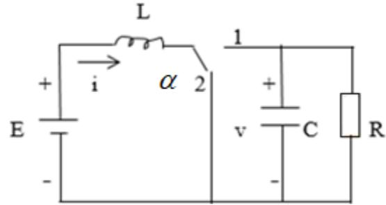
Fig. 1. A DC-DC boost power converter: the inductor  $L$ , load resistor  $R$ , capacitor  $C$ , input voltage  $E$ , switch position  $\alpha$ , inductor current  $i$  and capacitor voltage  $v$
