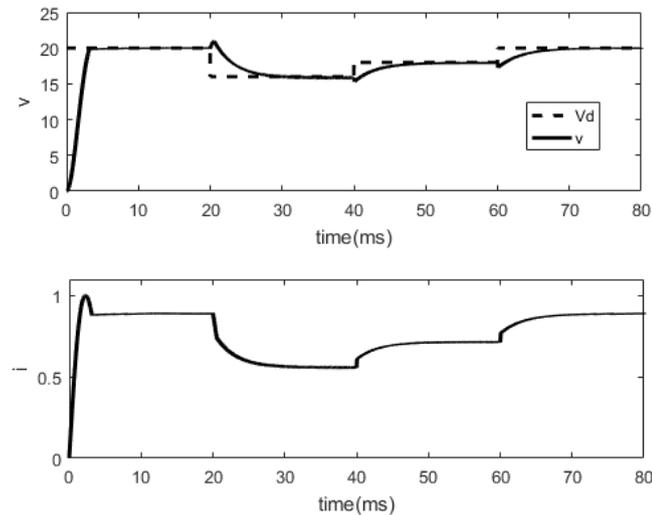
Fig. 3. The results of the PBC when  $V_d$  changes: the capacitor voltage  $v$  and inductor current  $i$
