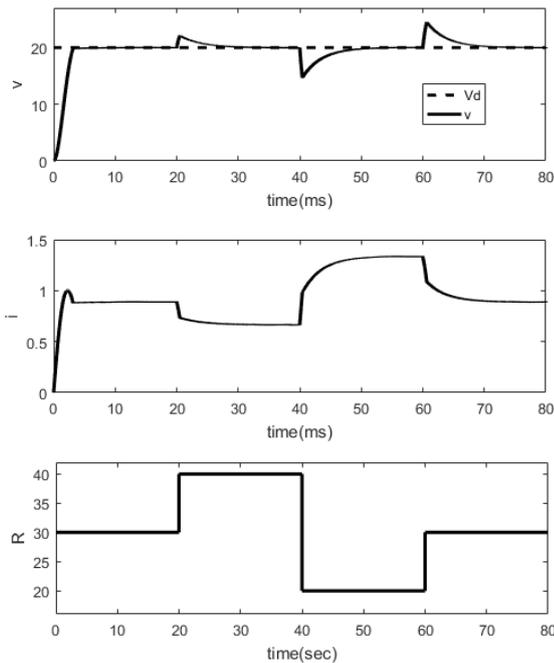
Fig. 6. The results of the PBC when  $R$  changes: the capacitor voltage  $v$  and inductor current  $i$  and load resistor  $R$
