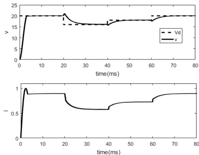
Fig. 4. The results of the SMC when  $V_d$  changes: the capacitor voltage  $v$  and inductor current  $i$
