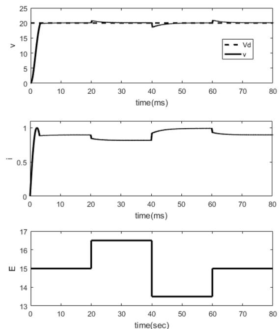
Fig. 10. The results of the SMC when  $E$  changes: the capacitor voltage  $v$  and inductor current  $i$  and input voltage  $E$
