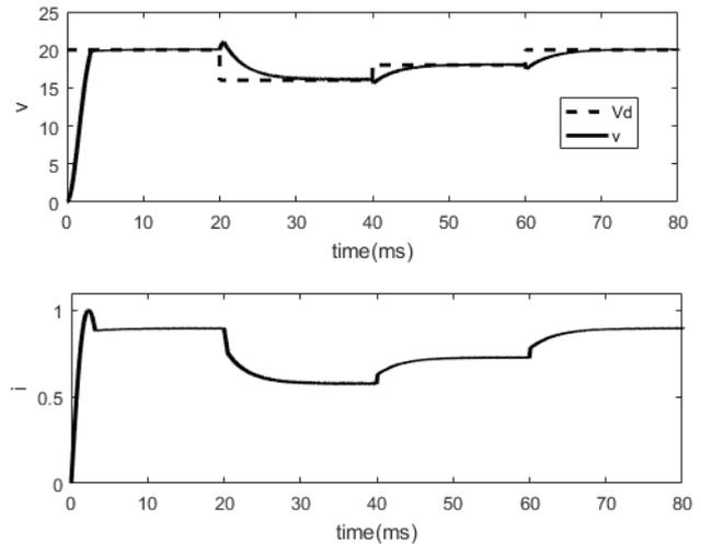
Fig. 5. The results of the PBC-SMC when  $V_d$  changes: the capacitor voltage  $v$  and inductor current  $i$
