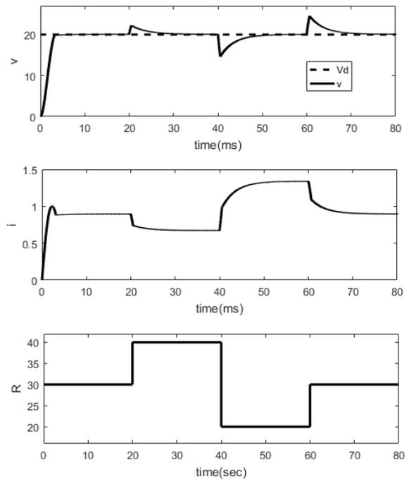
Fig. 8. The results of the PBC-SMC when  $R$  changes: the capacitor voltage  $v$  and inductor current  $i$  and load resistor  $R$
