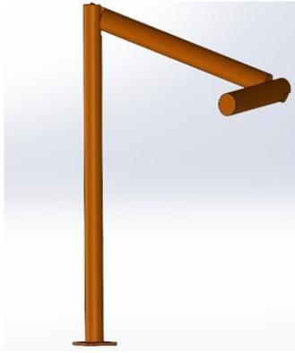
Fig. 7. Simplified SolidWorks model of the ABB IRB 140 robotic arm
