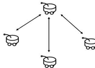
Fig. 3. Centralized architecture centered around a robot as the computing hub
