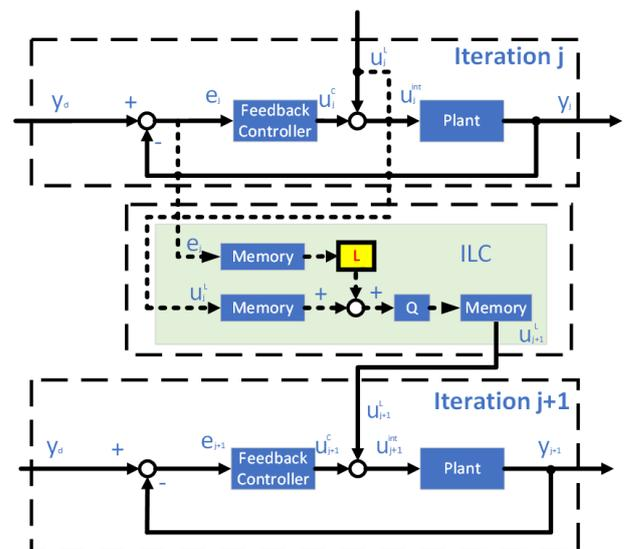
Fig. 7. Block diagram of the parallel ILC architecture
