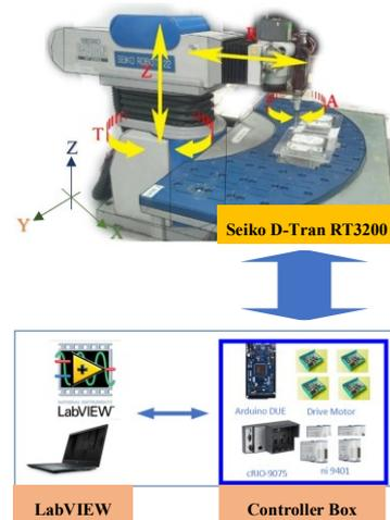
Fig. 4. Seiko D-Tran RT3200 and device for controller
