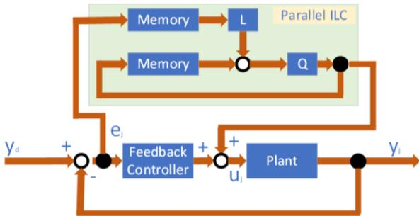
Fig. 5. Block diagram of Parallel ILC architecture
