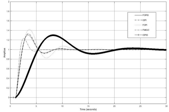
Fig. 35. Step response with gain variation for  $L = 0.1$  and  $T = 4$
