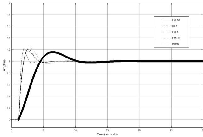
Fig. 33. Step response with gain variation for  $L = 0.1$  and  $T = 2$
