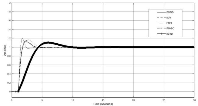
Fig. 31. Step response with gain variation for  $L = 0.1$  and  $T = 1.5$
