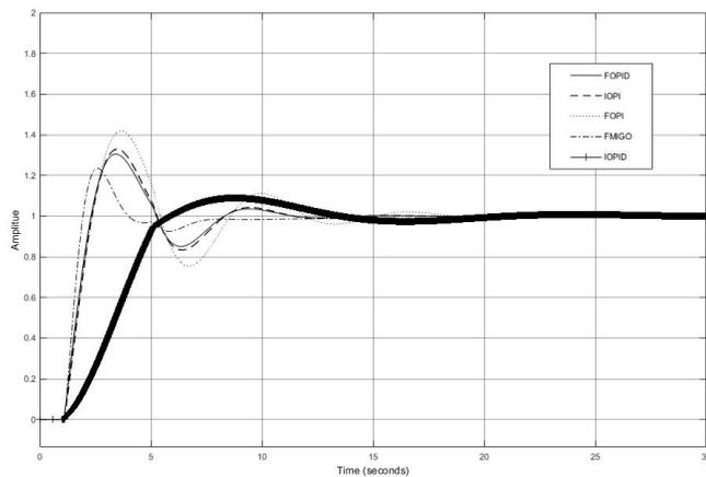
Fig. 34. Step response and load disturbance plot for  $L = 0.1$  and  $T = 4$
