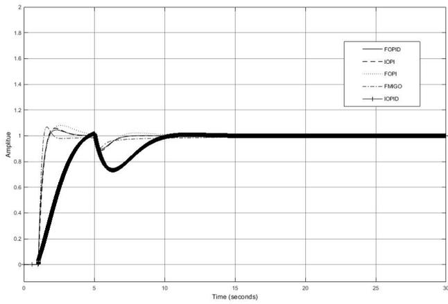
Fig. 20. Step response and load disturbance plot for  $L = 0.03$  and  $T = 1$
