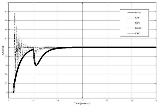
Fig. 26. Step response and load disturbance plot for  $L = 0.1$  and  $T = 0.3$
