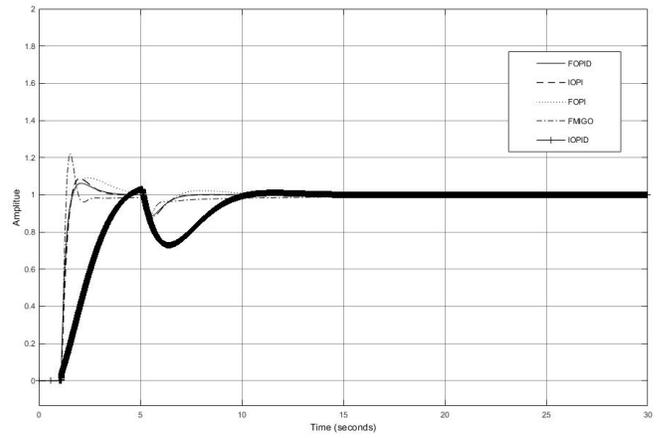
Fig. 24. Step response and load disturbance plot for  $L = 0.1$  and  $T = 1$
