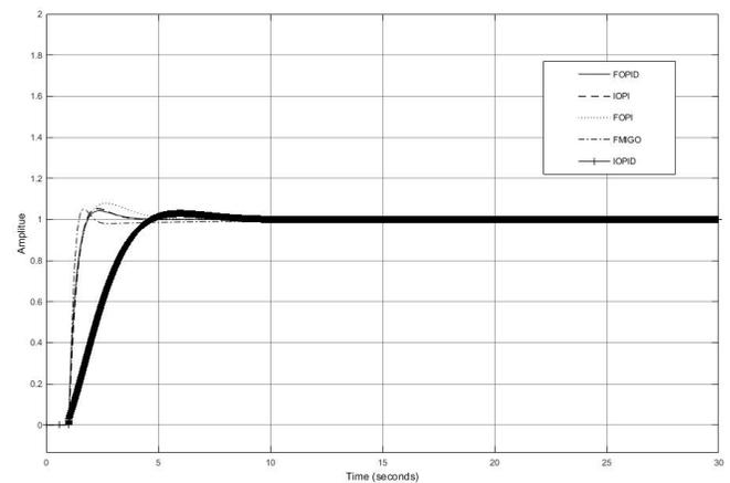
Fig. 19. Step response with gain variation for  $L = 0.01$  and  $T = 1$
