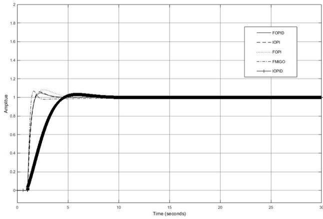
Fig. 21. Step response with gain variation for  $L = 0.03$  and  $T = 1$
