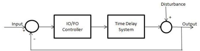
Fig. 1. Block diagram of IO and FO controllers with Time Delay System [2]
