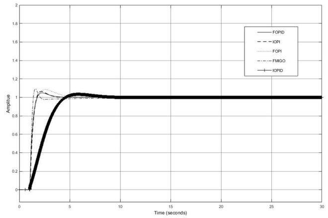
Fig. 23. Step response with gain variation for  $L = 0.05$  and  $T = 1$
