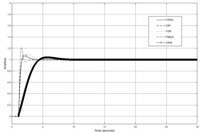
Fig. 25. Step response with gain variation for  $L = 0.1$  and  $T = 1$
