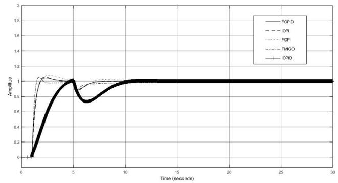
Fig. 18. Step response and load disturbance plot for  $L = 0.01$  and  $T = 1$
