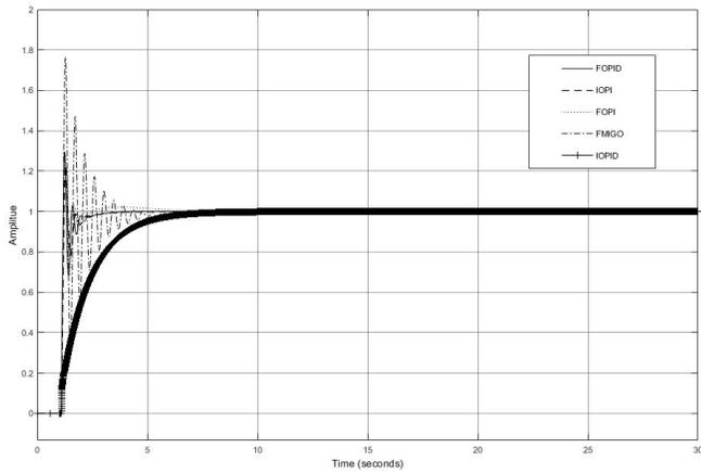
Fig. 27. Step response with gain variation for  $L = 0.1$  and  $T = 0.3$
