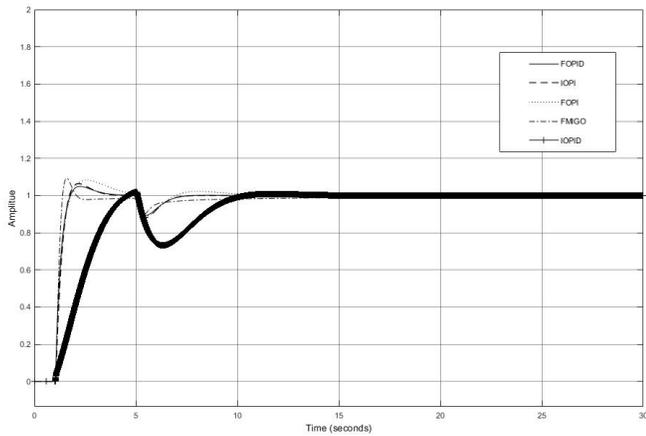
Fig. 22. Step response and load disturbance plot for  $L = 0.05$  and  $T = 1$
