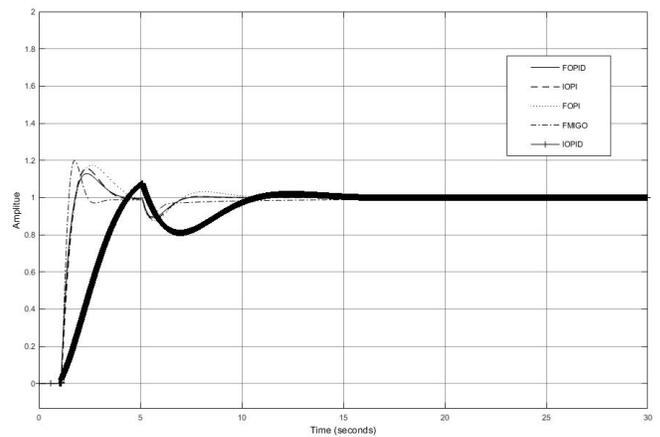
Fig. 30. Step response and load disturbance plot for  $L = 0.1$  and  $T = 1.5$
