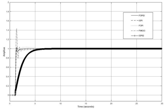
Fig. 29. Step response with gain variation for  $L = 0.1$  and  $T = 0.5$
