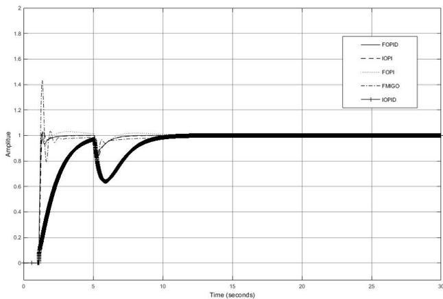
Fig. 28. Step response and load disturbance plot for  $L = 0.1$  and  $T = 0.5$
