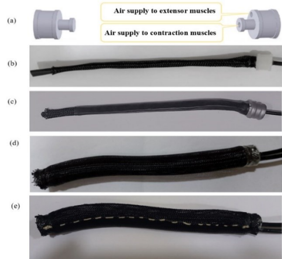
Fig. 15. Stages of CEB-PAM manufacturing: (a) The endcap design, (b) Connect CPAM to one of the endcaps, (c) CPAM is inserted into the bladder of EPAM, (d) Connect each CPAM and EPAM to the other endcaps and, (e) The actuator was sewn on one side
