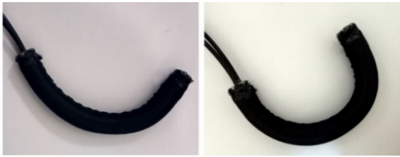
Fig. 16. The bending angle of CEB-PAM at various pressures for both CPAM and EPAM
