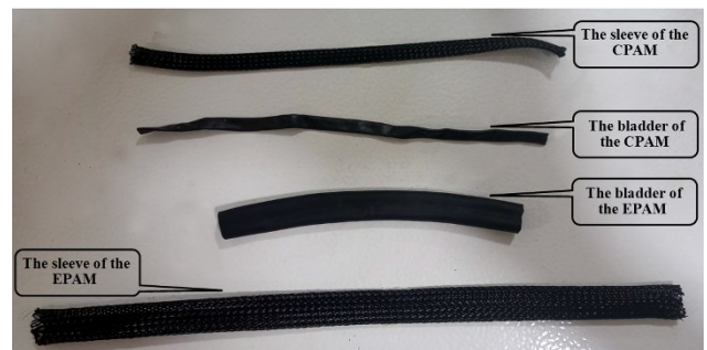
Fig. 7. The difference in the lengths of the bladders and sleeves of both the CPAM and EPAM
