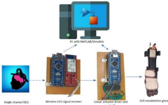
Fig. 2. Proposed hardware for the soft exoskeleton glove
