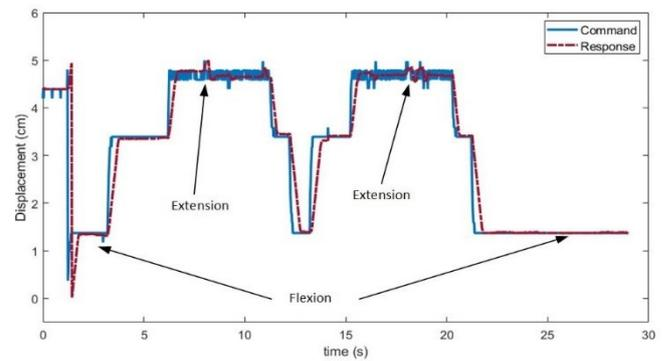
Fig. 10. Soft exoskeleton glove response to the commanded input signal from EEG
