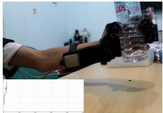
Fig. 11. Soft exoskeleton glove commanded using EEG signal
