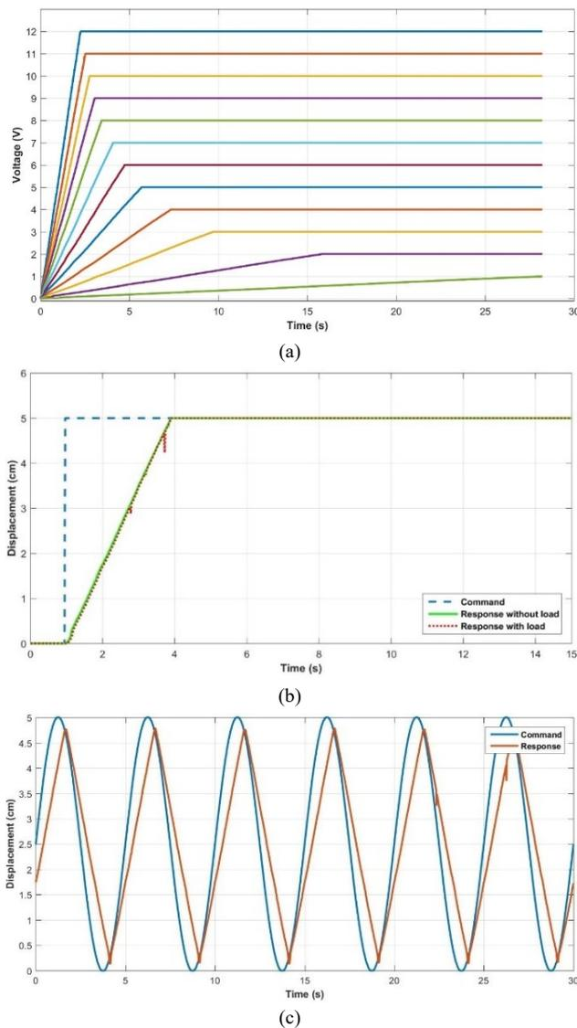
Fig. 9. Open-loop and closed-loop responses from the soft glove. (a) Voltage input signal variations to drive the linear actuator from 0 cm to 5 cm (full extension). (b) Response of the soft glove from the step input command. (c) Soft exoskeleton glove response to the sinusoidal commanded signal.
