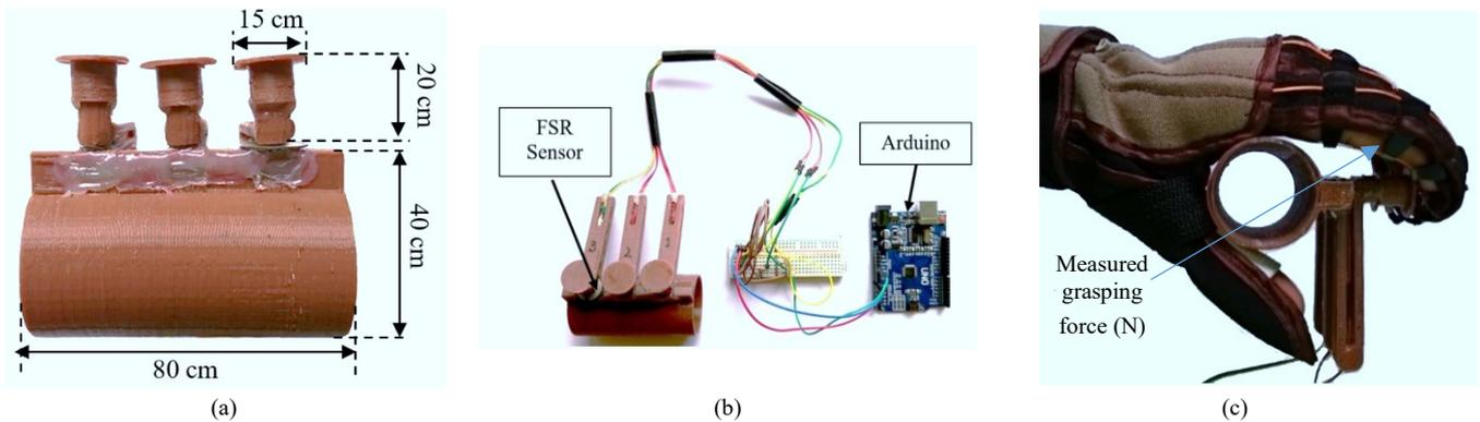
Fig. 6. Grasping force measurement. (a) Proposed grasping measurement. (b) Overall grasping measurement system. (c) Grasping force measurement
