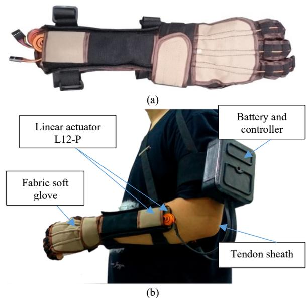
Fig. 1. Fabric-based soft exoskeleton glove, (a) Soft glove prototype, (b) The glove worn by a study participant
