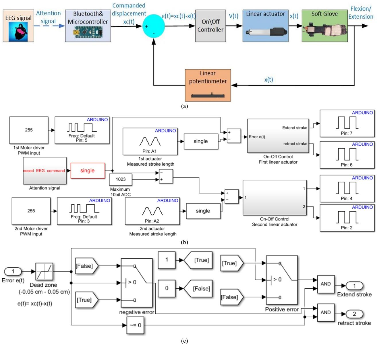
Fig. 4. Overall EEG control for soft exoskeleton flexion/extension motion assistance, (a) On-off control diagram block, (b) Embedded overall control on Arduino microcontroller, (c) Proposed on-off control on the soft glove motion
