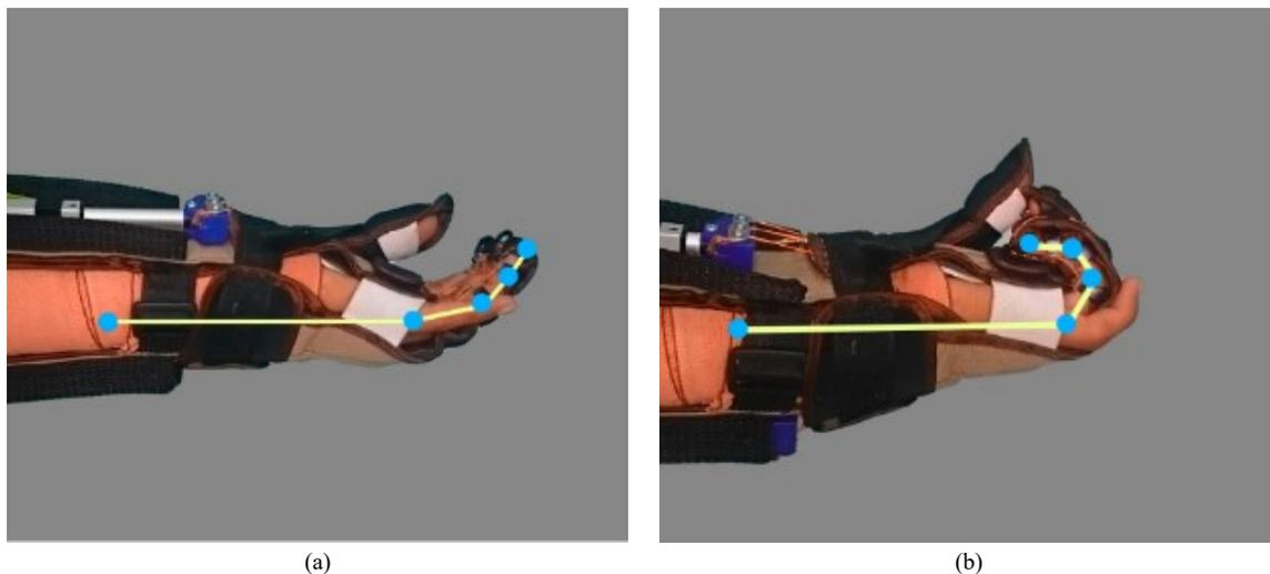
Fig. 5. Mechanical assistance for hand motion, (a) Finger extension, (b) Finger flexion
