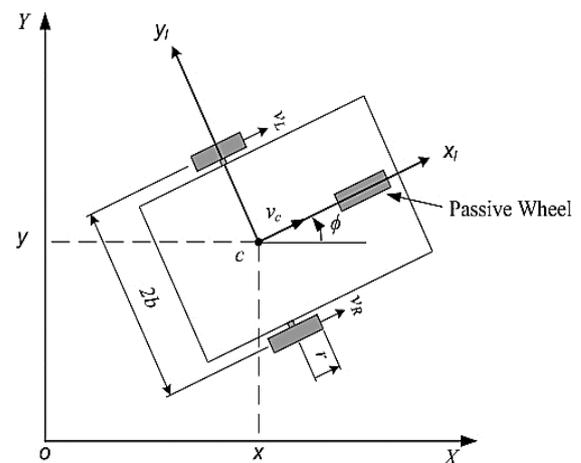
Fig. 1. Schematic model of mobile robot
