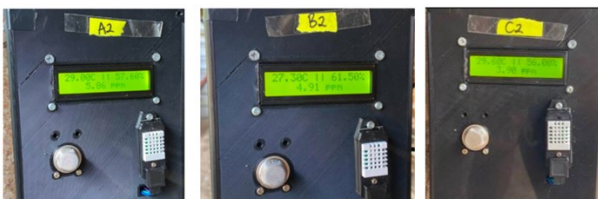
Fig. 14. LCD display of 3-parameter measurement results
