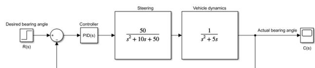
Fig. 2. Simplified block diagram for PID controller in self-guiding vehicle
