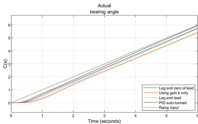
Fig. 8. Unit ramp response curves for self-guiding vehicle's bearing angle control
