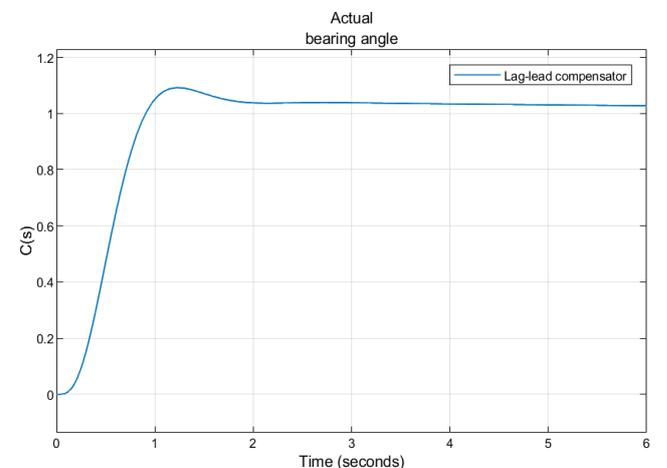
Fig. 5. The performance of lag lead compensation of self-guiding vehicle's bearing angle control
