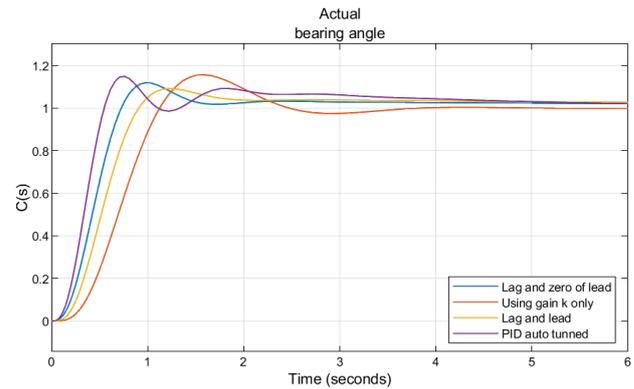
Fig. 7. Bearing angle controllers for self-guiding vehicles
