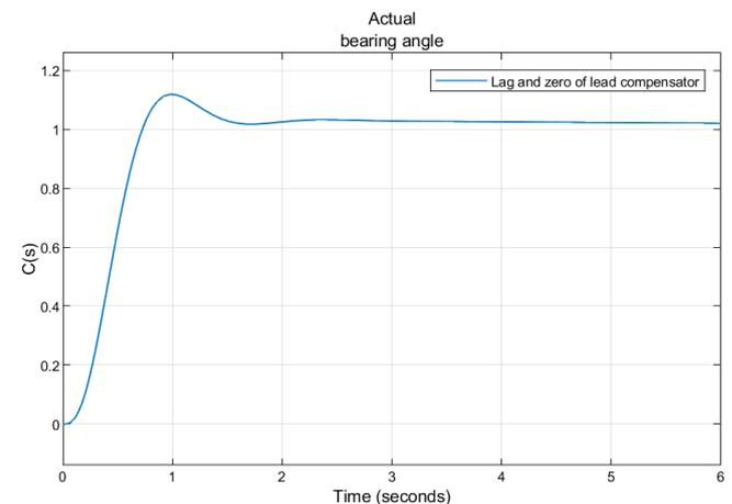
Fig. 4. The bearing angle control performance of a self-guiding vehicle using lag and zero of lead compensating
