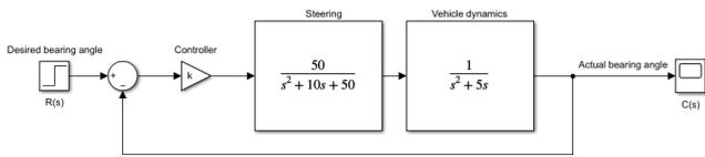
Fig. 1. Bearing angle control system in a self-guiding vehicle
