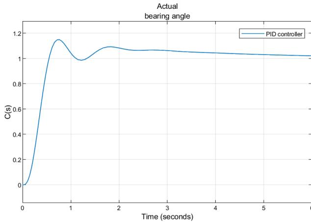
Fig. 6. Bearing angle control performance of a self-guiding vehicle using a PID controller
