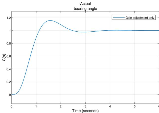
Fig. 3.  $k$  controller of self-guiding vehicle's bearing angle control
