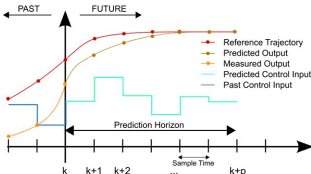
Fig. 7. MPC working principle [54]
