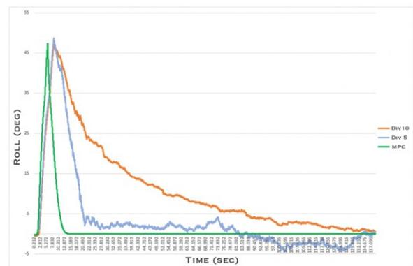
Fig. 10. OADCS simulation by MPC and PID
