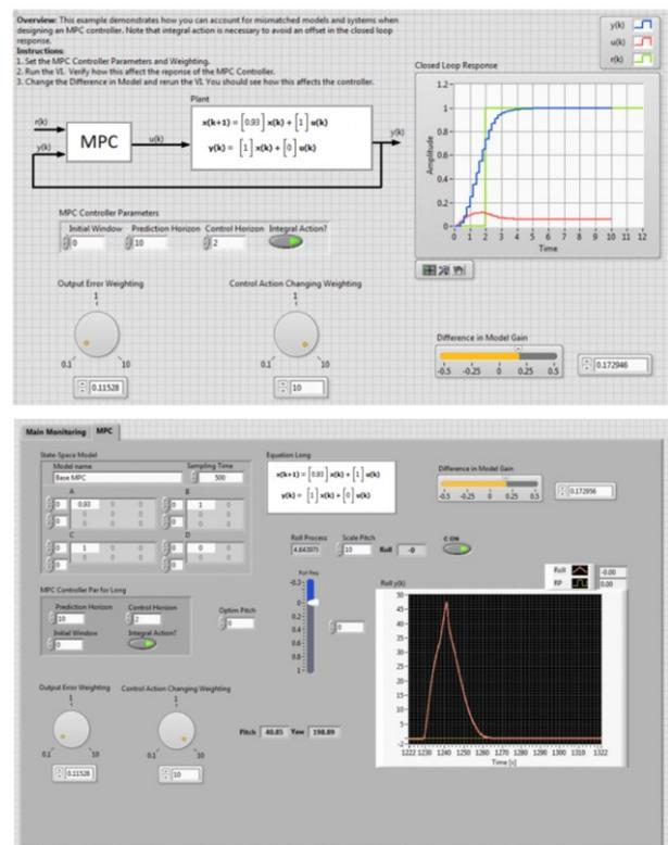
Fig. 9. MPC parameter settings and close loop program results
