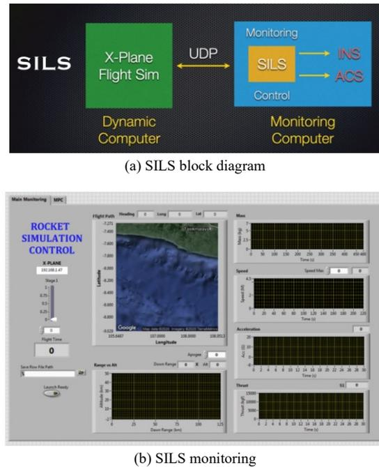
Fig. 5. SILS diagram and rocket simulation control window
