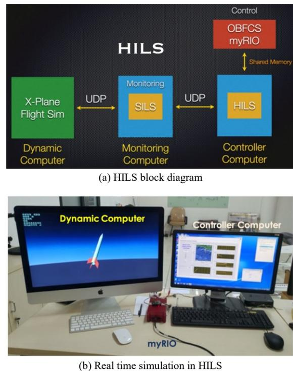
Fig. 6. HILS diagram and its simulation
