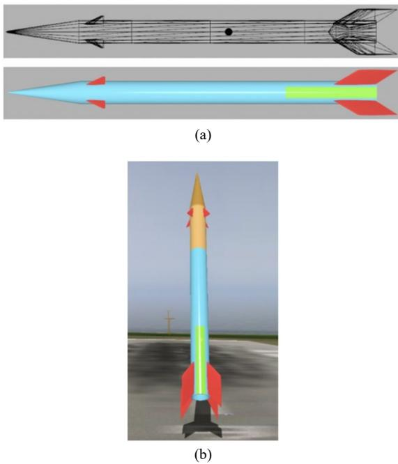
Fig. 4. The rocket model, augmented with an extra canard for managing the rocket's rotation, and the simulation
