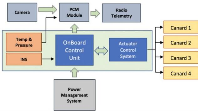
Fig. 2. OADCS block diagram which is fully controlled by NI myRIO module and LabView as the programming language
