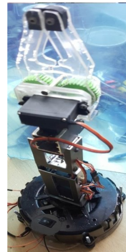
Fig. 9. The developed 5-DOF articulated robot arm
