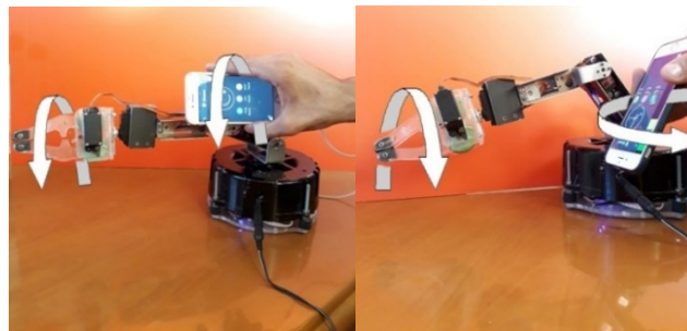
Fig. 17. End-effector rotates to the right and to left along the X axis
