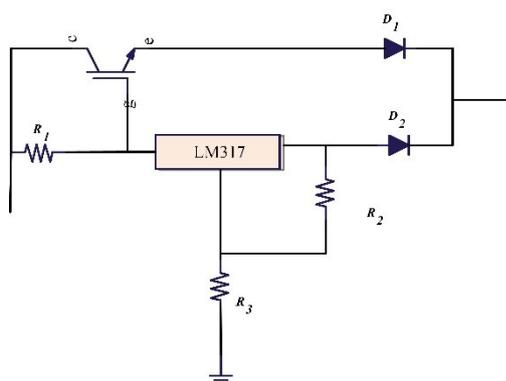
Fig. 15. The current booster circuit
