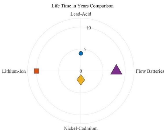
Fig. 8. Comparison of batteries life time
