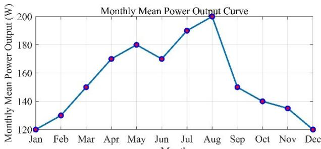
Fig. 17. The monthly mean power output of the studied system
