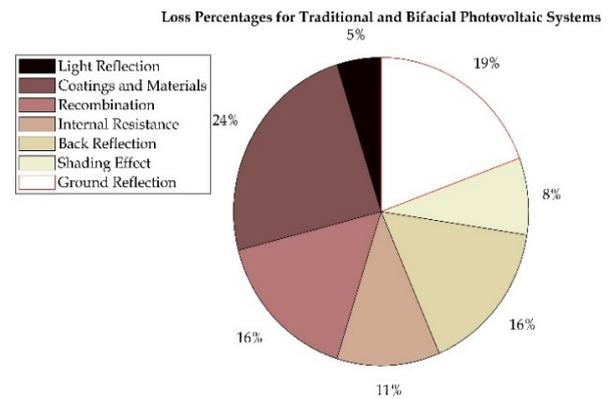
Fig. 2. The losses percentages for traditional and bifacial PV systems
