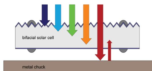
Fig. 3. Scheme of light passing through a bifacial solar cell and reflected back at the surface of a metal chuck
