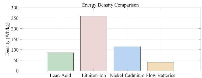
Fig. 10. Comparison of batteries energy density
