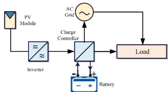
Fig. 13. The main components of the studied system
