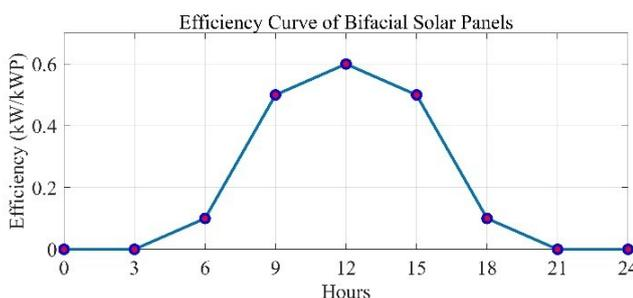
Fig. 18. The efficiency of bifacial PV panels
