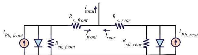
Fig. 16. The typical equivalent electrical circuit for a bifacial solar cell
