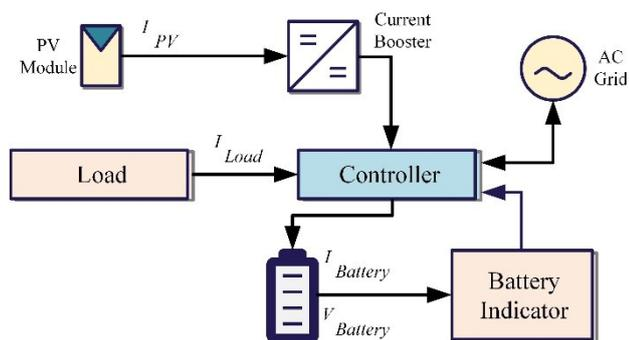
Fig. 14. The block diagram of studied system methodology
