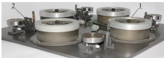
Fig. 2. Photograph of the platform without the top plate: 1 - four active one- or three-axis MR dampers; 2 - four elastic suspension nodes with quasi-zero stiffness
