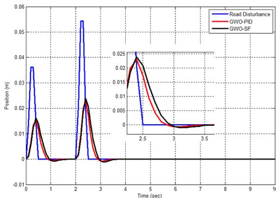
Fig. 12. Suspension system response when the mass of the car body increased by 20%
