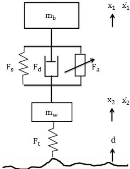
Fig. 1. Active suspension system
