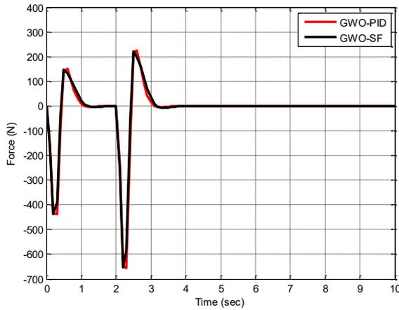
Fig. 11. Control law of the controllers when the mass of the car body increased by 20%
