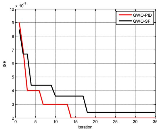
Fig. 8. GWO's convergence for the SF and the PID controllers
