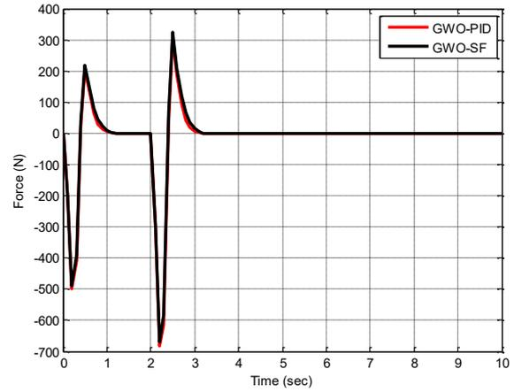
Fig. 13. Control law of the controllers when the mass of the car body decreased by 20%
