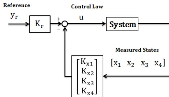
Fig. 3. The system with the SF controller
