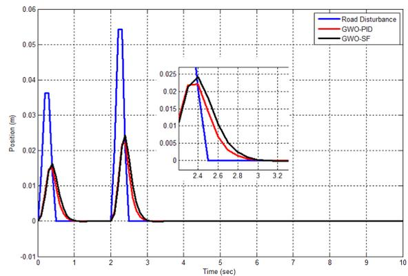
Fig. 14. Suspension system response when the mass of the car body decreased by 20%
