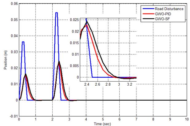
Fig. 10. Suspension system response
