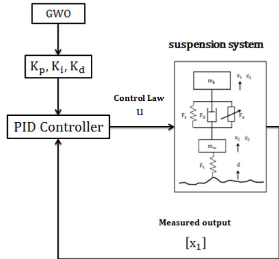
Fig. 6. Proposed PID controller tuned by GWO
