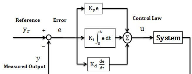
Fig. 2. The System with the PID controller
