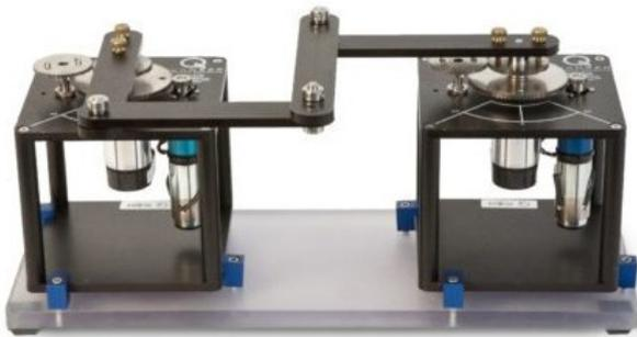
Fig. 6. Quanser's 2 DOF Robot model
