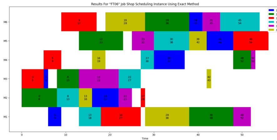
Fig. 5. Gantt chart for ft06 hypothetical manufacturing using exact method
