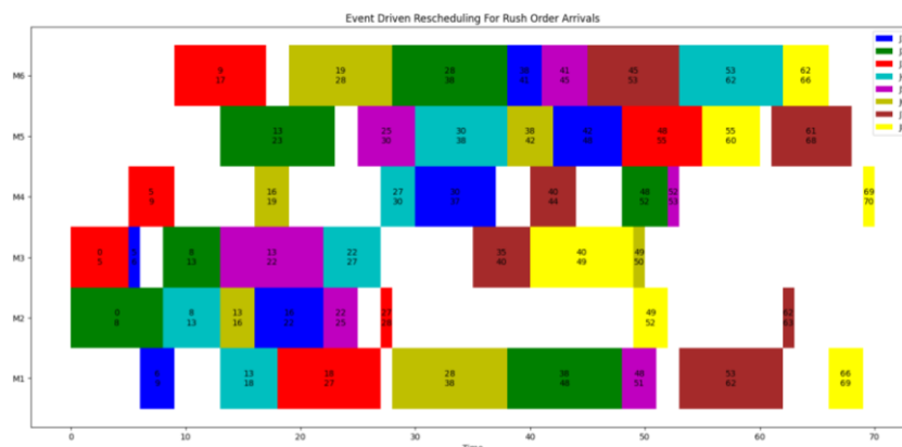
Fig. 19. Event-driven rescheduling for hybrid bike and electric bike arrival at t=30 and t=40
