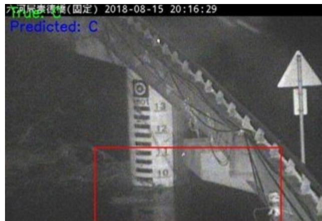
Fig. 11. Normal water level detection - class C prediction
