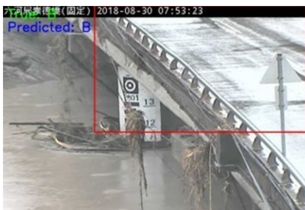
Fig. 10. Rising water level detection - class B prediction
