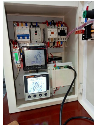
Fig 3. The cabinet with the Modbus_Ethernet Communication System for Collecting, Storing Data, and Monitoring Electrical Power Consumption, Temperature, and Humidity Parameters
