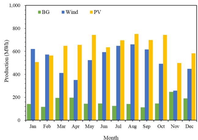
Fig. 12. Power output of the generating PV/Wind/BG/Battery throughout the year
