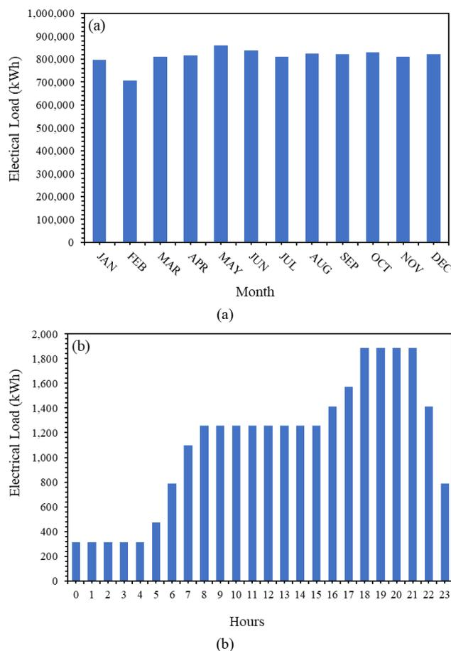
Fig. 2. (a) Electrical month load profile, (b) Electrical hours load profile
