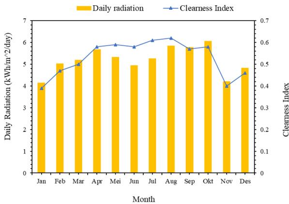
Fig. 5. Solar radiation and clearness index for the West Waru Village [58]
