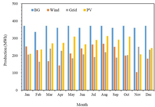
Fig. 11. Power output of the generating PV/Wind/BG/Grid throughout the year
