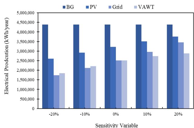
Fig. 13. Effect of scaled sensitivity variables on Electricity Production
