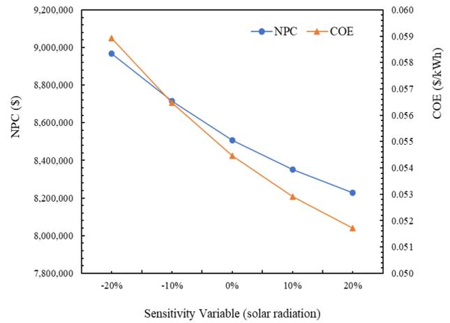
Fig. 18. Variation of NPC and COE with solar radiation
