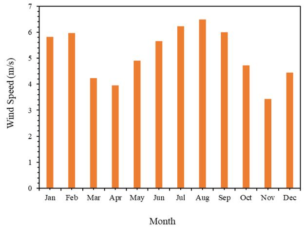
Fig. 7. The average monthly wind speed for the site at 10 m [58]
