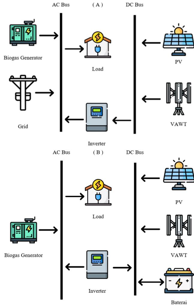
Fig. 10. Proposed configurations for two scenarios of the hybrid renewable energy system: (a) On-Grid, (b) Off-Grid
