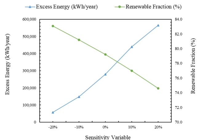
Fig. 14. Effect of scaled sensitivity variables on renewable fraction and excess energy
