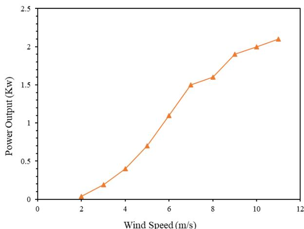
Fig. 8. Wind turbine power curve EN-2KW-H [63]
