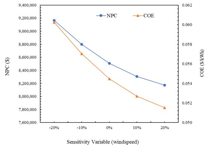
Fig. 19. Variation of NPC and COE with wind speed
