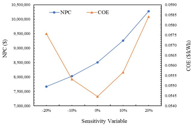
Fig. 15. Effect of scaled sensitivity variables on NPC and COE
