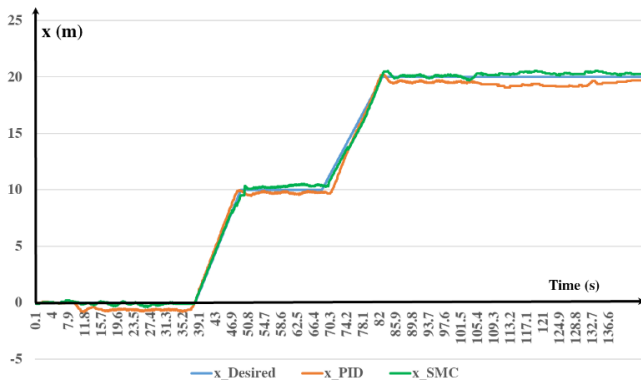
Fig. 15. The position of the quadcopter in the x direction corresponds to three cases: desired trajectory, PID-controlled trajectory, and sliding mode control trajectory
