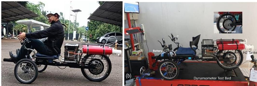
Fig. 7. (a) Outdoor and (b) Indoor test of the new platform trike
