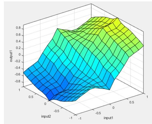
Fig. 7. Surface viewer of triangular membership outputs
