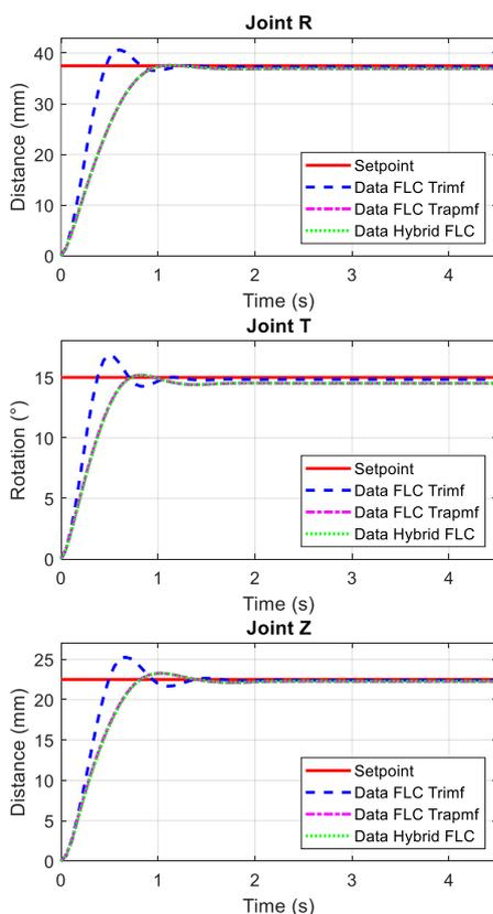
Fig. 14. Analysis of system response for setpoints at joints R, T, and Z, respectively, 37.5, 15°, and 22.5
