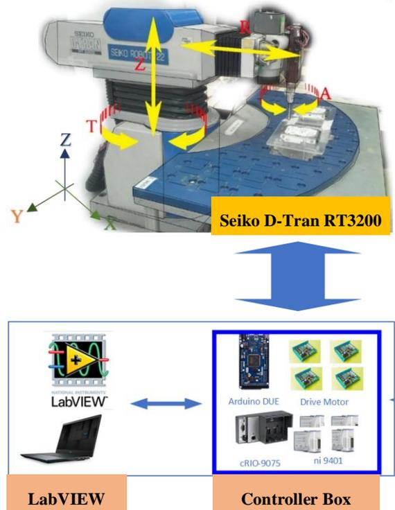
Fig. 2. Controller Integration for Seiko D-Tran RT3200
