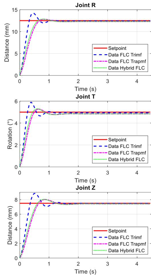
Fig. 13. Analysis of system response for setpoints at joints R, T, and Z, respectively 10, 3.75, and 5
