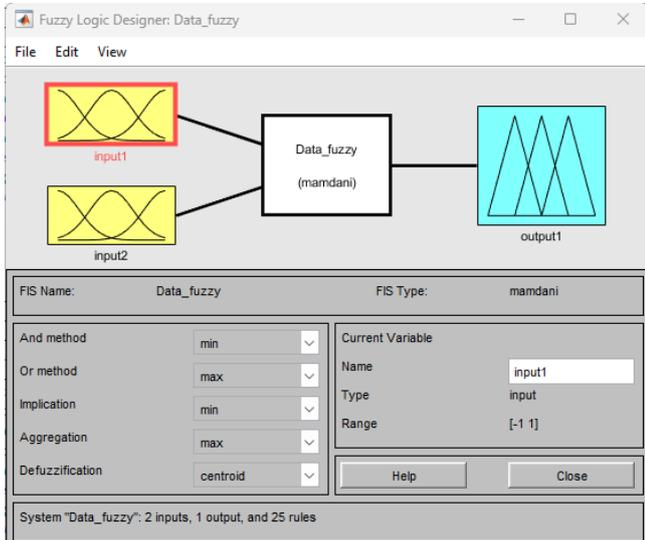
Fig. 5. Fuzzy logic designer for system configuration
