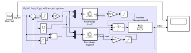
Fig. 12. Simulink implementation of the hybrid fuzzy-expert system
