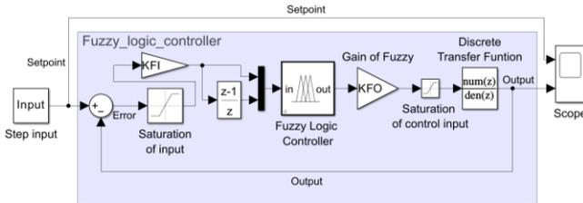
Fig. 10. Simulink model for fuzzy logic system
