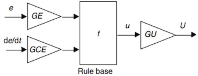
Fig. 4. Fuzzy PD controller framework
