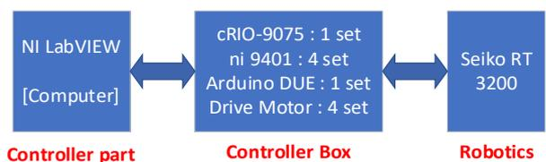
Fig. 3. Complete system block diagram for seiko D-Tran RT3200
