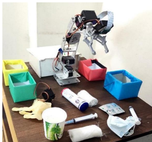
Fig. 4. Voice-controlled, ROS-based robotic arm
