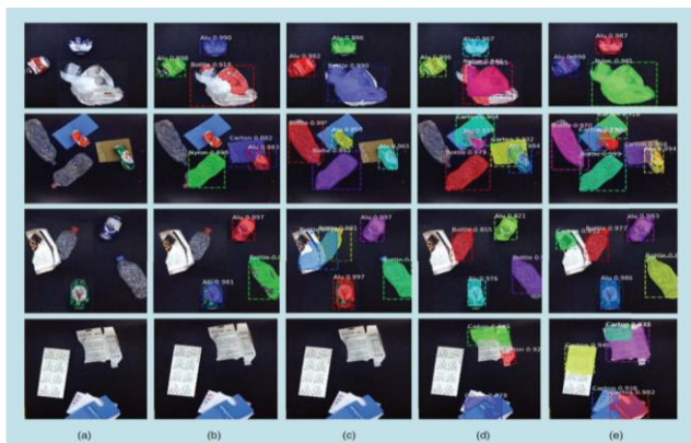
Fig. 7. Material sorting using R-CNN mask where the colors of different debris are randomly selected
