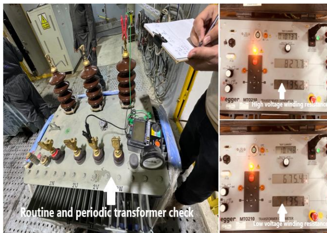
Fig. 3. Shows part of the tests conducted on a real model of a 1000 kVA transformer to determine the resistance values of the coils
