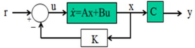
Fig. 3. Block diagram of LQR closed-loop control system
