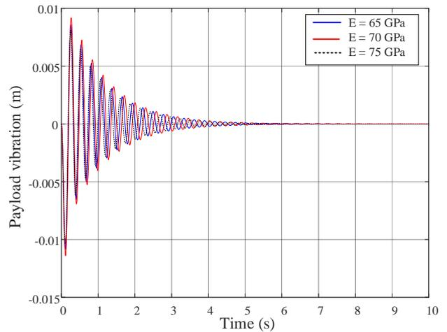
Fig. 10. Robustness of the proposed controller under the variation of the material properties
