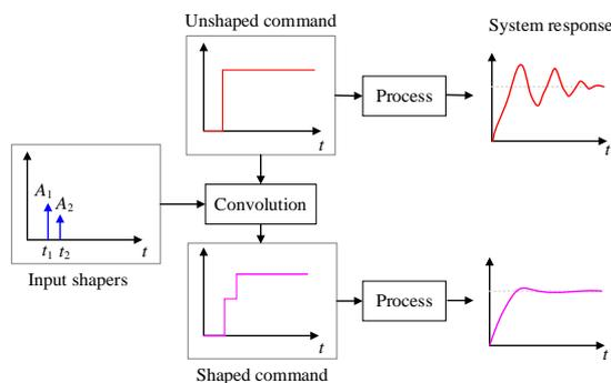
Fig. 3. Input shaping control
