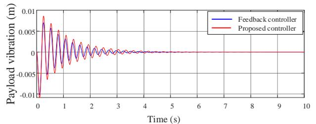
Fig. 11. Comparison of the proposed controller with the feedback control
