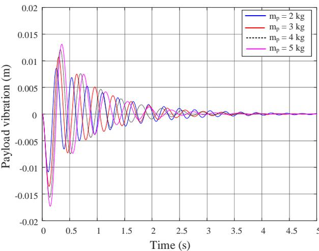
Fig. 9. Robustness of the proposed controller under the variation of the payload mass
