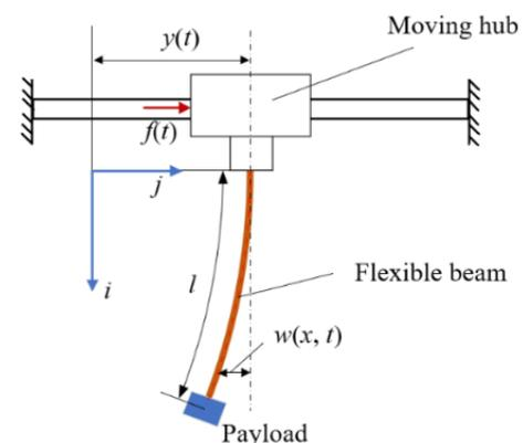
Fig. 2. System of a flexible beam attached to a moving hub
