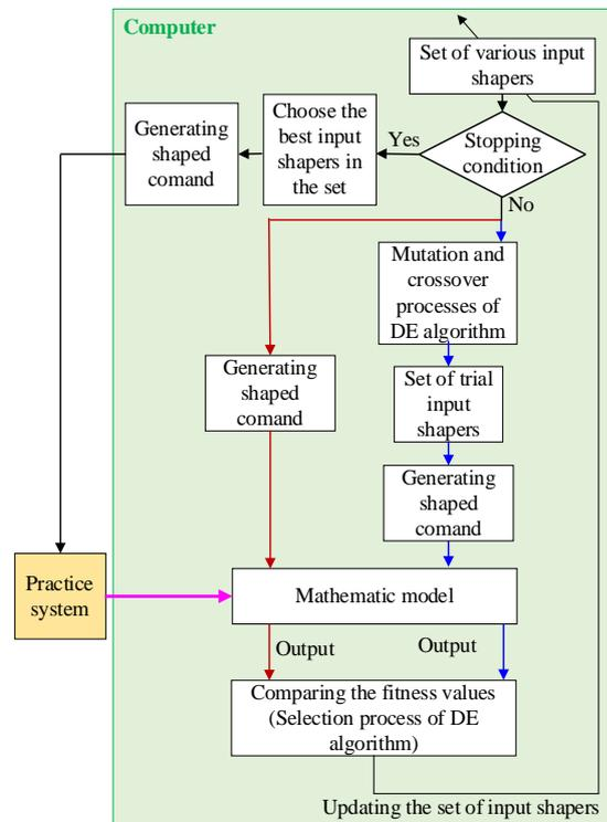
Fig. 4. The control scheme is based on input shaping and differential evolution methods
