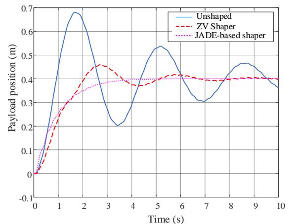
Fig. 6. Response of the payload position (i.e.,  $y(t) + w(l, t)$ )
