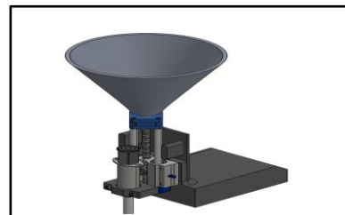
Fig. 8. Dosing system for liquid fertilizers
