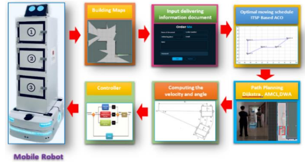
Fig. 3. The working procedure of the document delivering mobile robot
