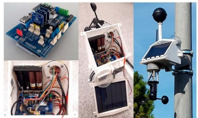
Fig. 8. Solar-powered transmitter box integrating multiple environmental sensors for continuous outdoor monitoring
