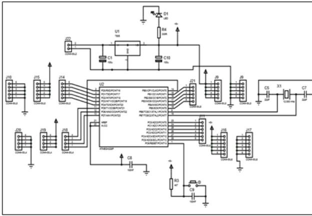
Fig. 3. Minimum system schematic diagram
