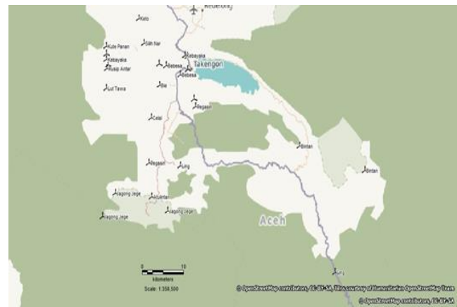
a. The placement of existing towers, 30 towers with a total of 90 bts
