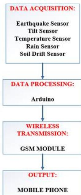
Fig. 1. General block diagram of the system.
