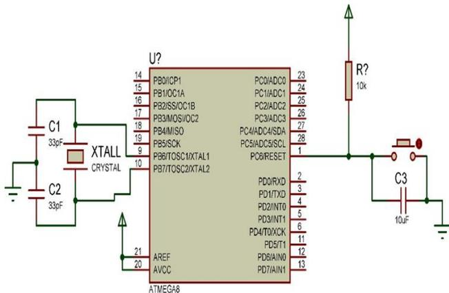
Fig. 5. Minimum system schematic
