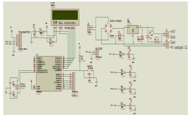
Fig. 6. Transmitter device schematic
