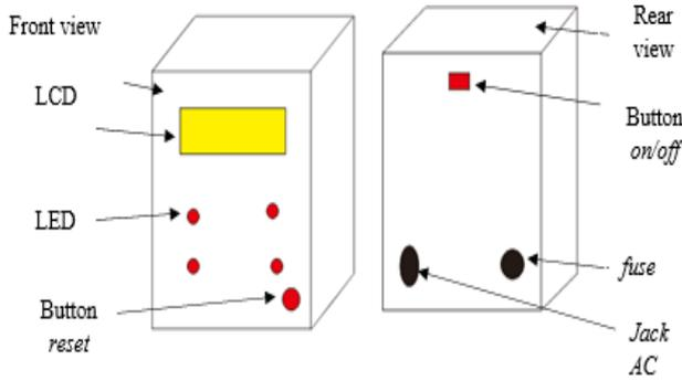
Fig. 4. Receiver device visualization
