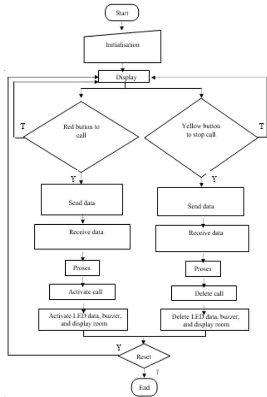
Fig. 2. System work flow chart
