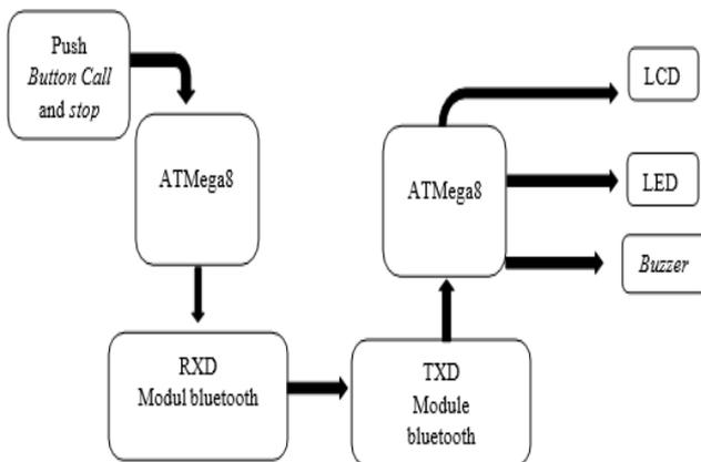
Fig. 1. System components
