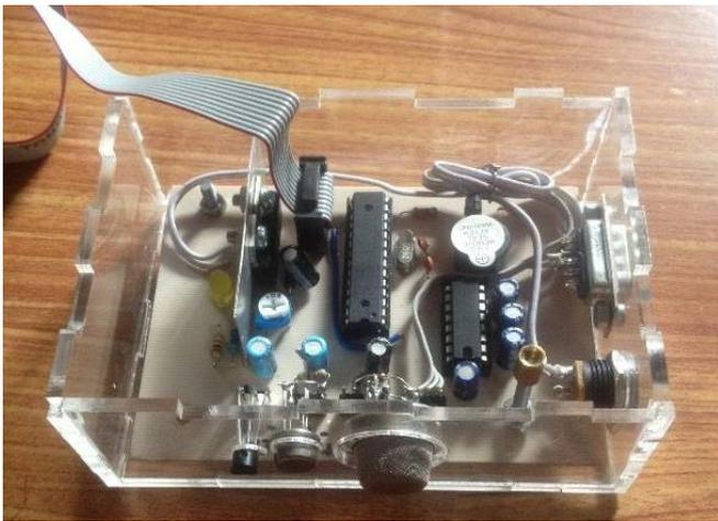
Fig. 4. A prototype of a Fire Detection Device
