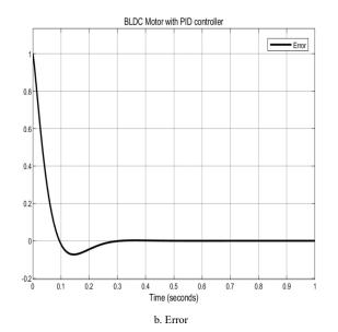
Fig. 13. Simulation response of the motor with PID control
