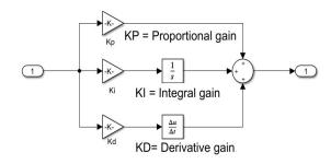
Fig. 5. PID controller
