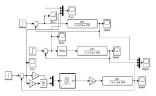
Fig. 4. Model of BLPMDC motor without a controller, with PID controller, and with FLC
