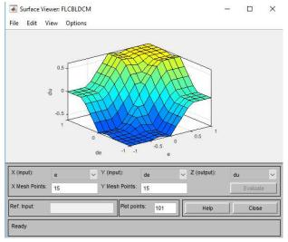
Fig. 11. The FLC-Surface viewer of input (e, de) & output (du)
