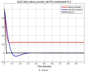
Fig. 15. Simulation response of the motor without the controller, with PID controller, and with FLC
