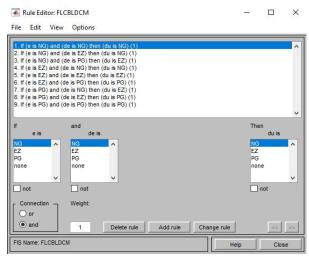
Fig. 9. FLC-Rule Editor of input (e, de) & output (du)
