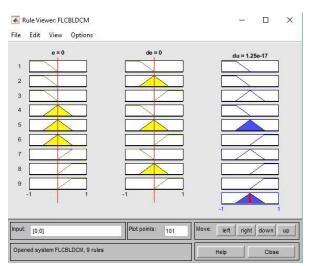
Fig. 10. FLC-Rule viewer of input(e,de) &output(du)
