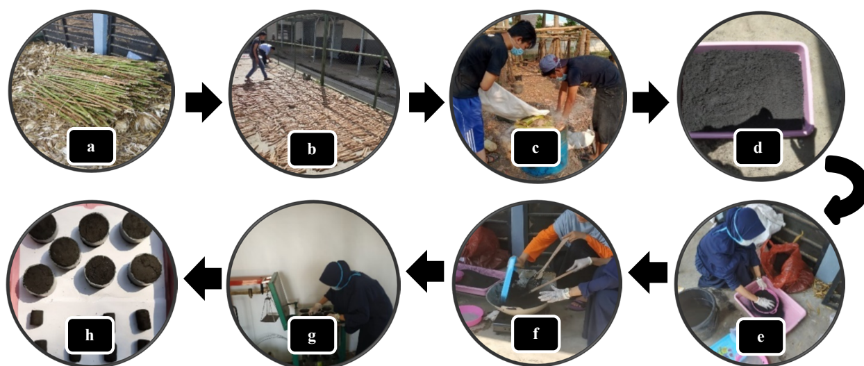
Figure 1. The production process of agricultural waste briquettes: a. Fresh tobacco stem waste; b. Drying tobacco stem; c. Charcoal process; d. Charcoal of several agricultural wastes; e. Charcoal sifting process; f. Briquette process; g. Press machine; h. Briquette
