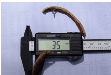
Figure 1. Bark thickness measurement using digital caliper
