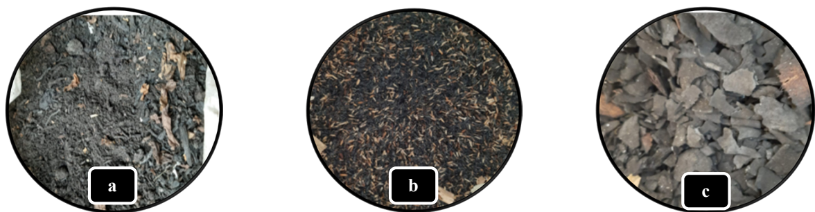
Figure 3. Raw material of briquette waste: a. Tobacco stem and leaf charcoal; b. Rice husk charcoal; c. Coconut shell charcoal
