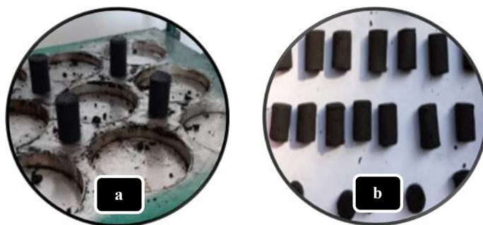
Figure 4. a. Pressing briquette; b. Briquette size, 2.25 cm x 3.25 cm
