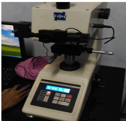
GAMBAR 3. Microhardness vickers test
