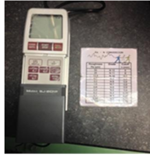
GAMBAR 5. Roughness tester (a) unit roughness tester (b) display control
