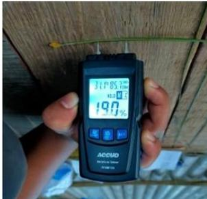
Gambar 5. Pengukuran kadar air awal lidi sawit
