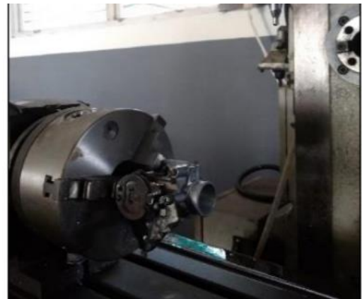
Gambar 6. Proses pembesaran throttle body
