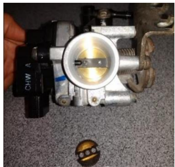
Gambar 7. Penggantian coin butterfly
