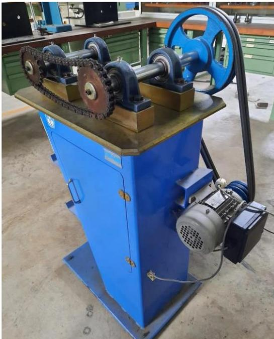
GAMBAR 2. Sprocket and Chain Alignment Kit
