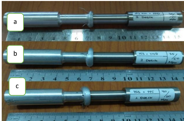
Figure 4. CDFW welding results (a) 30 MPa, (b) 35 MPa, (c) 40 MPa
